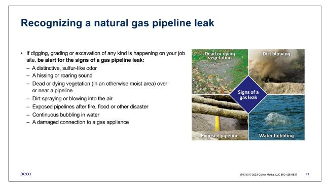
Recognizing a natural gas pipeline leak. It is important to learn the warning signs.
